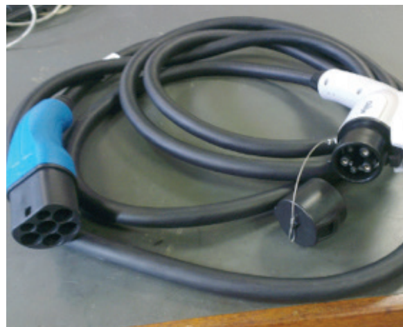
Type 2 (top) and Type 1 (bottom) charging cables
