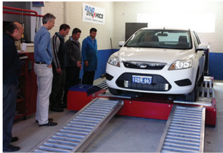
Dynamometer testing of electric Focus prototype at Polytechnic
