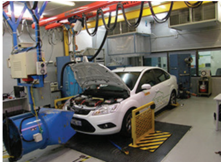
Dynamometer range testing of electric Focus at Orbital Engines (Wäger)
