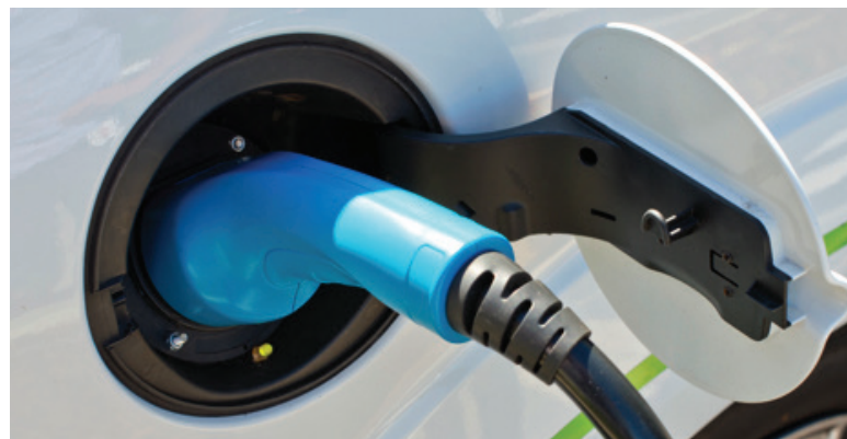
Converted Ford Focus with IEC 62196-2, Type 2, Gen. 2 ‘Mennekes’ vehicle inlet
