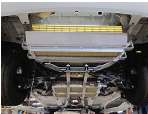
Batteries under the vehicle
