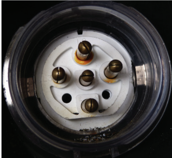
Original three-phase vehicle inlet with rust marks
